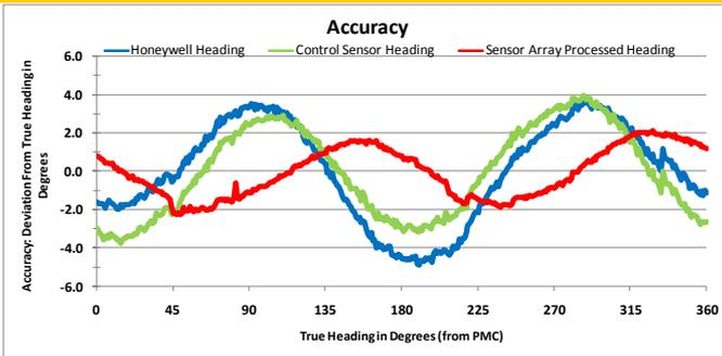
It was determined that multiple sensors working together can indeed increase the precision, accuracy, and repeatability of the system. The graph above shows the accuracy across 360 degrees. The table below shows the overall improvements in each of these areas. This shows that this type of implementation is very feasible and could potentially lead to more accurate digital compasses in the near future.
