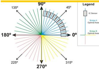
Here the orientation of IO sensors spread evenly across 0-90 degrees is shown. This leads to optimal axes which are distributed across the entire 360 degree spectrum, at 9 degree intervals.
