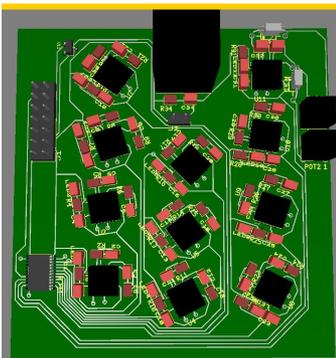
To the left is a 3-dimensional representation of the daughter board. The daughter board hosts a total of 11 sensors, 10 oriented in the fashion discussed above, and one additional sensor at 0 degrees as a control. Each sensor also includes a power LED and RC networks for scaling if necessary. The single control sensor has adjustable range via the potentiometers.
